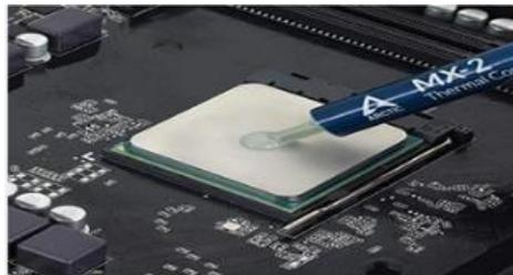
**Fig. 3.9: Thermal Paste**
