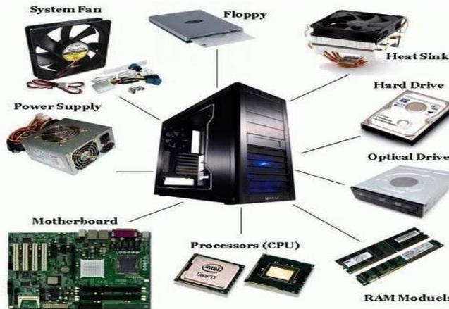
**Fig. 1.28: Common Parts in Computer system**
