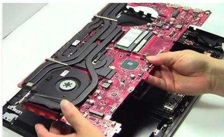
Fig. 2.10: Motherboard Being Removed
