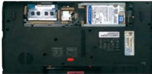
**Fig. 5.3: Remove screws from the hard drive and disconnect it**
