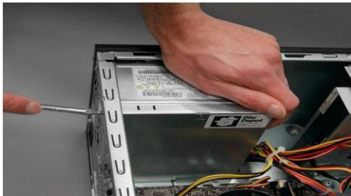
**Fig. 3.16: Install the Power Supply**
