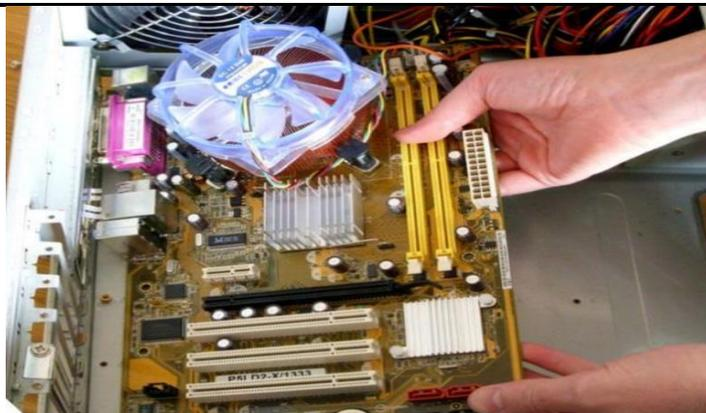
**Fig. 3.22: Motherboard install**
