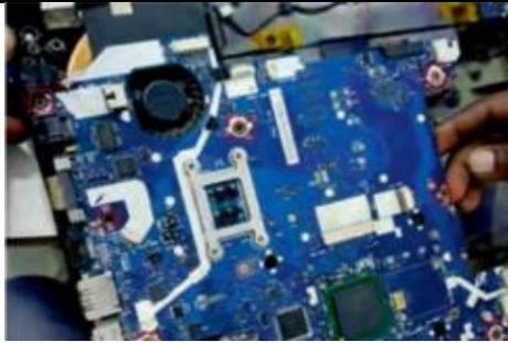
**Fig. 5.14: Disconnect cables from motherboard and remove screws**
