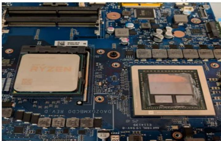
**Fig. 3.6: Socket CPU in a laptop**
