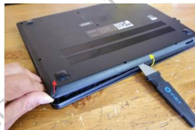
**Fig. 2.13: Reassembling the Laptop**
