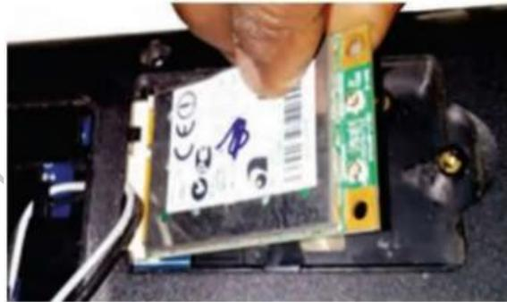
**Fig. 5.13: Disconnect Wi-Fi Module**
