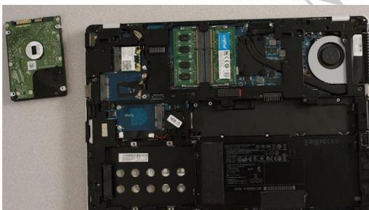
**Fig. 4.21 Locate and Remove Old Drive**
