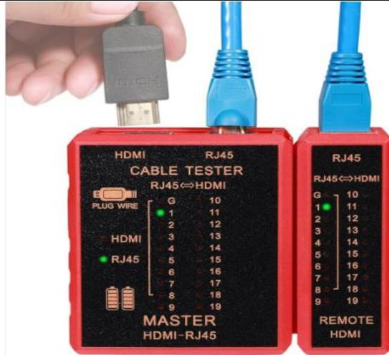
**1.22 Testing for USB, HDMI, or other ports**
