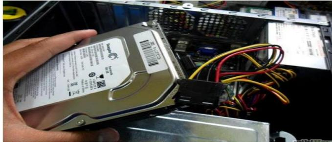
**Fig. 3.32: SATA cable connect HDD**
