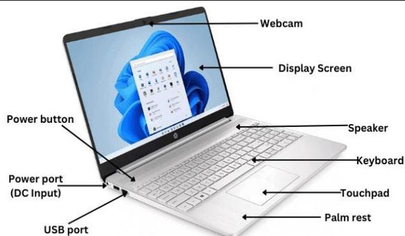
**Fig. 1.22: External components of Laptops**
