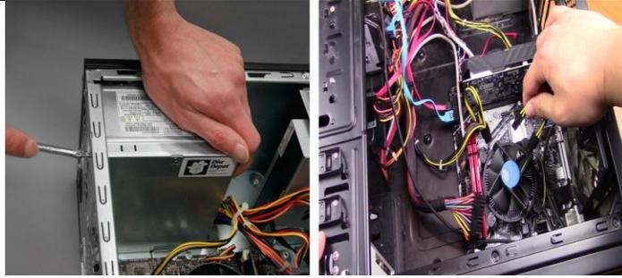
**Fig. 3.31: Remove Connector**
