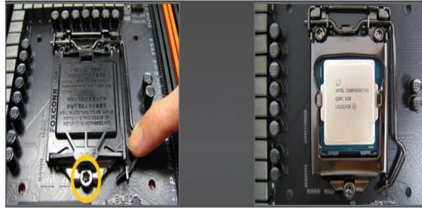
**Fig. 3.12: Protective socket cover**
