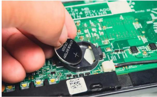
**Fig. 2.15: CMOS Battery**
