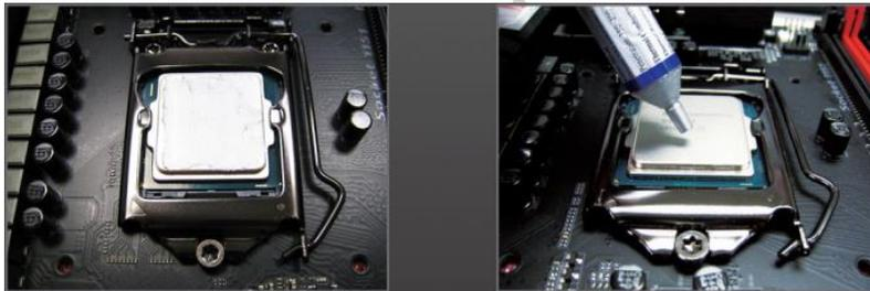
**Fig. 3.13: Heat sink paste surface in CPU**
