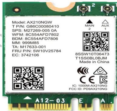
**Fig. 1.39: Wireless Network Adapter**
