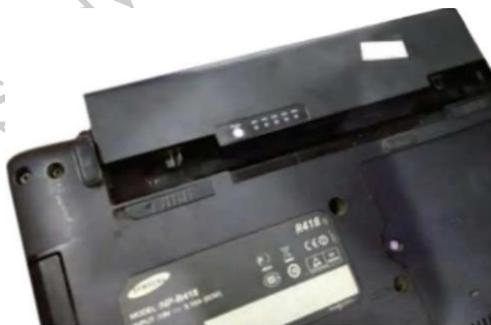
**Fig. 5.1: Remove battery**
