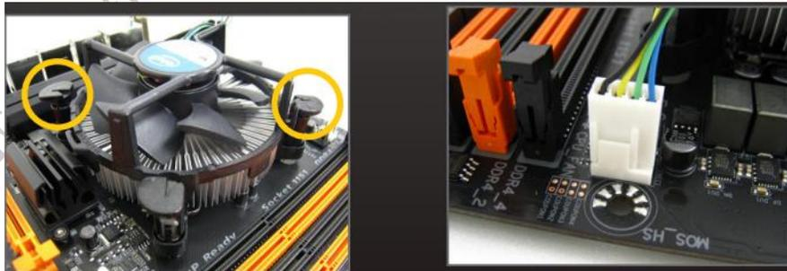
**Fig. 3.14: CPU\_FAN connector in CPU**
