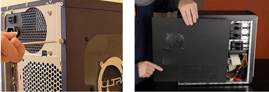
**Fig. 3.28: Case First Remove the Screws**
