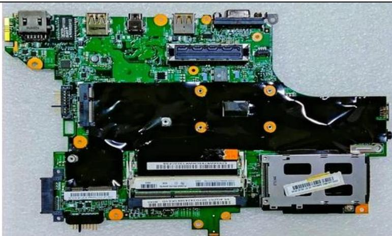
**Fig. 3.5: Laptop motherboard with an integrated CPU**
