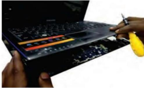
**Fig. 5.2: Separate palm rest from bottom case**
