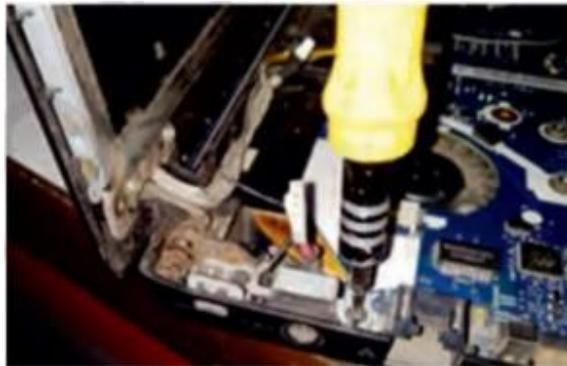
**Fig. 5.12: DC power jack mounted under display hinge**
