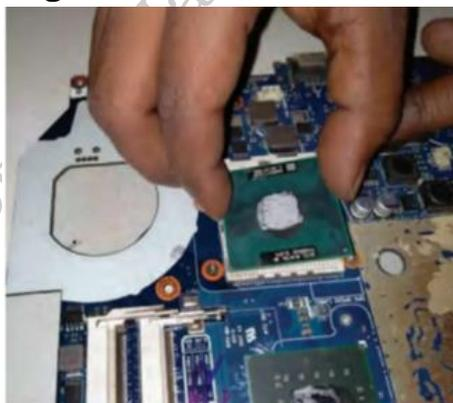
Fig. 5.19: Fit processor in the socket
